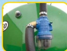
Secondary trap ensures maximum pump protection
