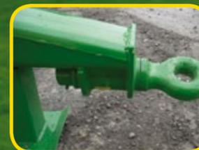
Swivel hitch and sprung drawbar are standard on recessed tanks
