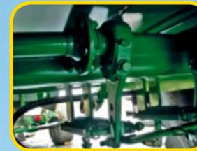
Recessed tanks come with strong 30mm brake rams and 1/2" brake hydraulic hose
