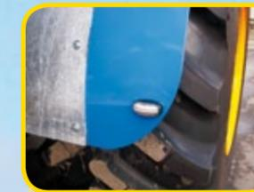
Fully recessed tanks come with LED lights on the mudguards
