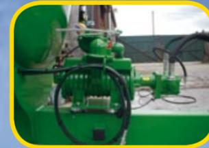
Hydraulically driven pump
