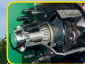
Recessed tanks bigger than 1800 Gallon come with ADR commercial axles and 420 x 180 brake shoes
