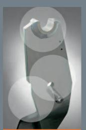
**SUPER STRONG SUBFRAME.** Quicke's Delta subframe has extraordinarily heavy-duty dimensions with many contact surfaces, all featuring precision work. Details such as the 60 mm wide U support and 40 mm locking pin enable the loader to cope with difficult and heavy jobs for many years.
