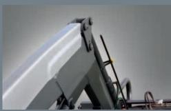
**COMPACT IMPLEMENT INDICATOR.** The position indicator is compact so that it doesn't stick up and cause damage or become damaged itself. It is easy to fit and can be adjusted in three positions for various implements, ensuring exact precision of the implement's angle with the ground.
