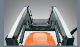
**SIGHT-OPTIMISING DESIGN.** No pipes or hoses that restrict your view. No dirt or rubbish that can accumulate, even if you fit extra equipment to your loader. These are the obvious advantages with Q Vision, where all pipes and hoses are protected in the loader arm.
