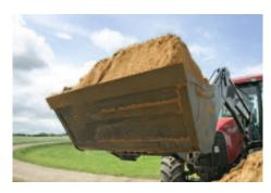
Naturally it has been our aim to design and produce a bucket that does not allow spillage. What is the point of having a large volume bucket if you cannot fill it properly, or if material spills out of it? Therefore our buckets have sides that are laser-cut. The result is a bucket design where the rear edge and the front edge in particular are especially high. It is now possible to fill the bucket completely. You have complete control of the material, and the bucket does not spill any material.
