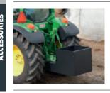
The counter-weight improves the stability of the tractor/loader unit. Connection and disconnection is simply done using the attached coupling shaft.
