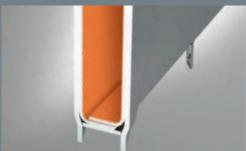
**KNEE PLATE.** Cross-section of the loader arm by the knee bracket. The loader arm's double C profile is here strengthened with a knee plate.
